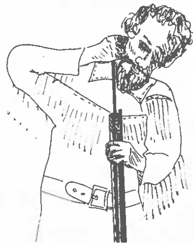
Seat ball on powder with ramrod
