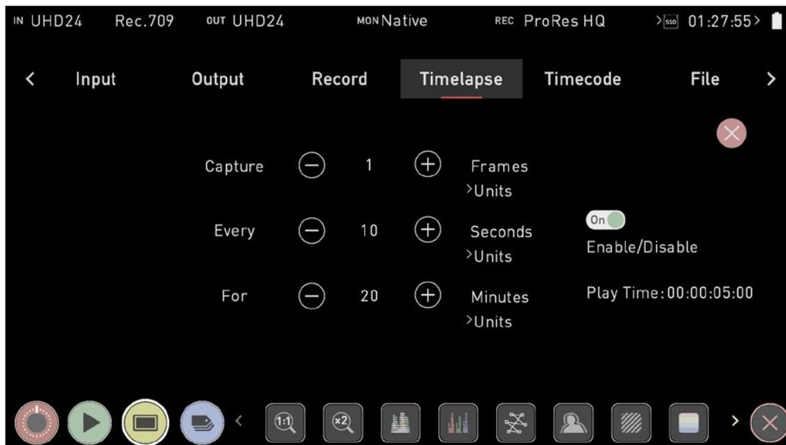
This menu allows you to set up recording of a time-lapse sequence as a single video file in ProRes, DNx or ProRes RAW from an HDMI or SDI source.
