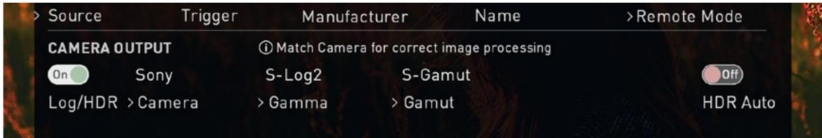
Now you are ready to capture Log and simultaneously use ATOMOS 10 image processing to preview the final HDR result in the field, rather than dealing with the washed out look of Log for critical exposure decisions.
