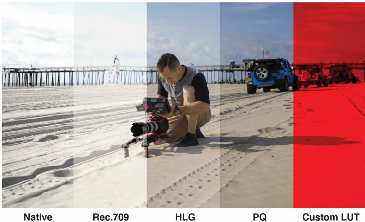
The main impact of HDR is apparent in the specular highlights and bright areas. The areas that would have previously been 'blown out' will now contain visible detail and information to enhance your content. HDR provides more headroom allowing you to show more detail. Experimentation with increased exposures is encouraged.
