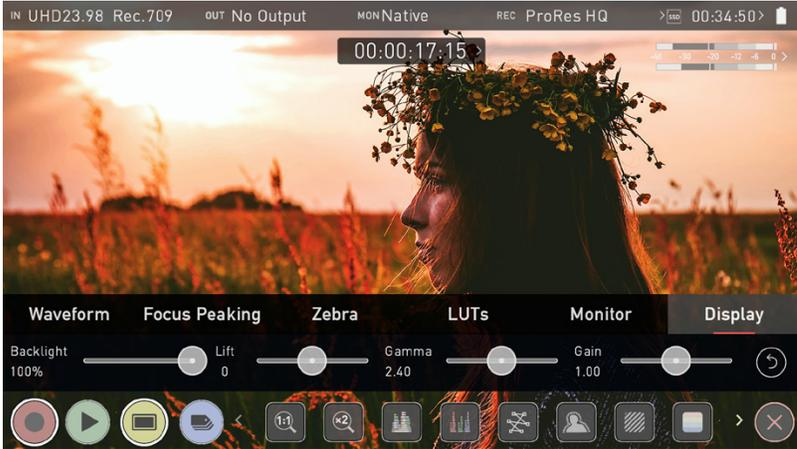
With this mode selected you have the option to change the screen brightness by adjusting the slider when in Native mode. At 100% brightness, the image will be using the full 3000nit peak brightness of the display. As with any electronic screen device, increasing the brightness will increase the power draw and battery life will be effected accordingly. Adjustments can also be made to the Lift, Gamma and Gain of the display.
