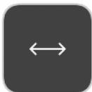
Allows you to de-squeeze images when monitoring content filmed with anamorphic lenses. Tap the de-squeeze icon to cycle through the options to select the amount of de-squeeze required, so that the image on your SHOGUN STUDIO 2 is not distorted.
