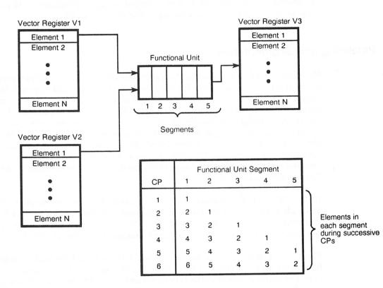
Figure 2-11. Segmentation and Pipelining Example
