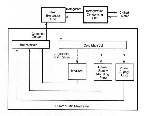
Figure 1-5. CRAY Y-MP Mainframe Cooling System
