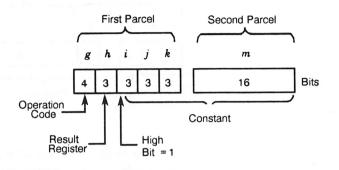
Figure 2-24. 2-parcel Instruction Format for a 24-bit Immediate Constant with Combined i, j, k, and m Fields
