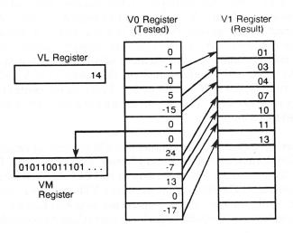
Figure 2-18. Compressed Index Example
