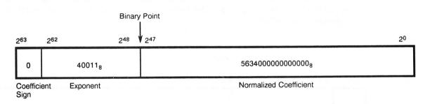
Figure 2-6. Internal Representation of Floating-point Number
