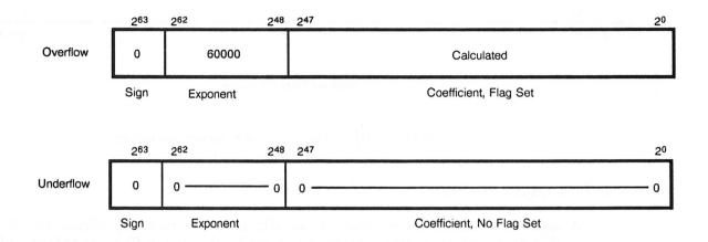
Figure 2-8. Floating-point Add and Multiply Range Errors
