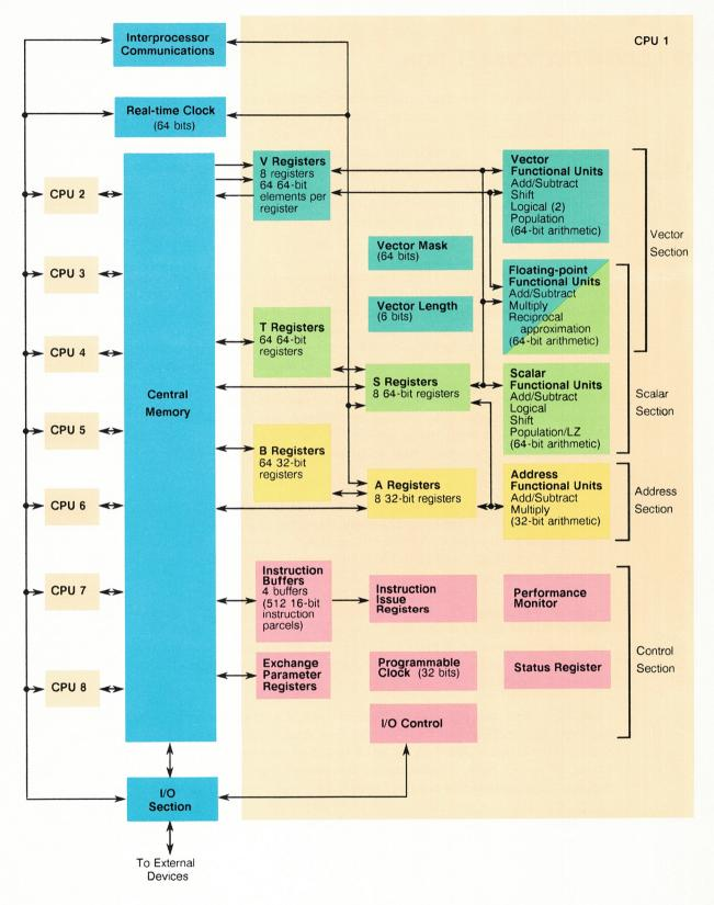
Figure 2-1. 8-processor CRAY Y-MP Computer System Block Diagram
