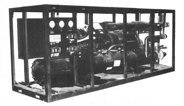
Figure 1-6. Refrigeration Condensing Unit
