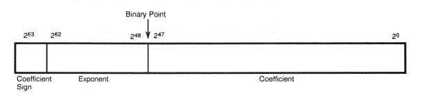
Figure 2-5. Floating-point Data Format
