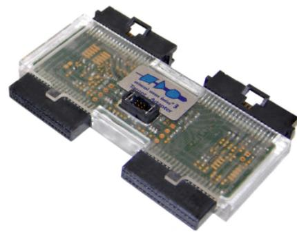
The UAD3 Multi AURIX Debug Adapter is an adapting solution and extension for the Universal Access Device 3+ (UAD3+). It enables **synchronized debugging of AURIX™ multi-chip systems** with two tightly coupled AURIX™ MCUs (e.g. Infineon's Automotive Ethernet Gateway Evaluation Board) in one single debug session. The UDE® Multi AURIX debug solution ensures **synchronous stop, single step and restart** as well as **synchronized suspend** of peripherals.
