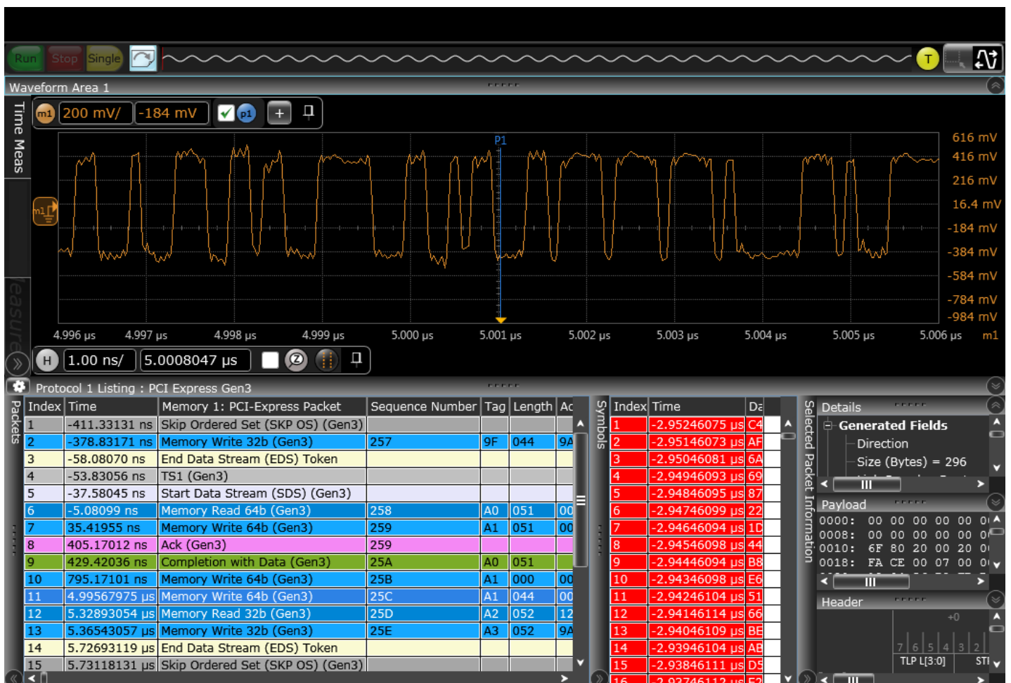
UXR-Series 25 GHz 4-channel model decoding PCI Express Gen 3 packets.
