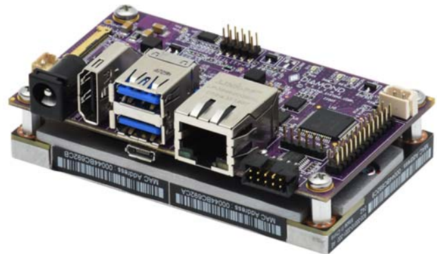
ZiggyBox internal electronics showing bottom-mounted Jetson TX2/TX2i Module
