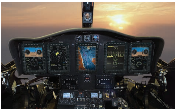
The Rockwell Collins Avionics Management and Display System aboard the S-92 Sikorsky helicopter is among the INTEGRITY-178 applications approved as compliant to DO-178B Level A, the most stringent safety assurance level for avionics software.
