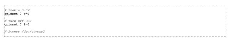
Nimbelink modules require settings for the specific modems. Verify in the datasheet of the modem appropriate for your cell network to determine if the module uses USB. If not, verify the expected serial baud rate and settings. Some modems need 3.3V power, and some modems expect a typical of 4V.
