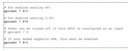
**Note:** Some Nimbelink cell modems have a long startup and may not show up on USB for a minute before enumerating on USB.
