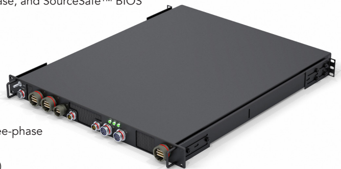
TITAN-1U Conduction-cooled with 38999 mil-circular connectors
