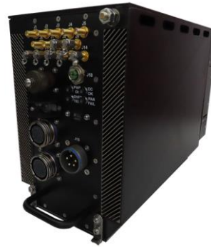
This is the chassis after nickel plating, painting, and addition of the front I/O panel.
